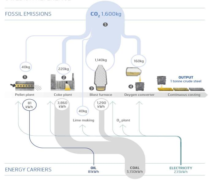
Principal system description. Numbers do not reflect a specific production site or time period. All numbers per tonne of crude steel.
